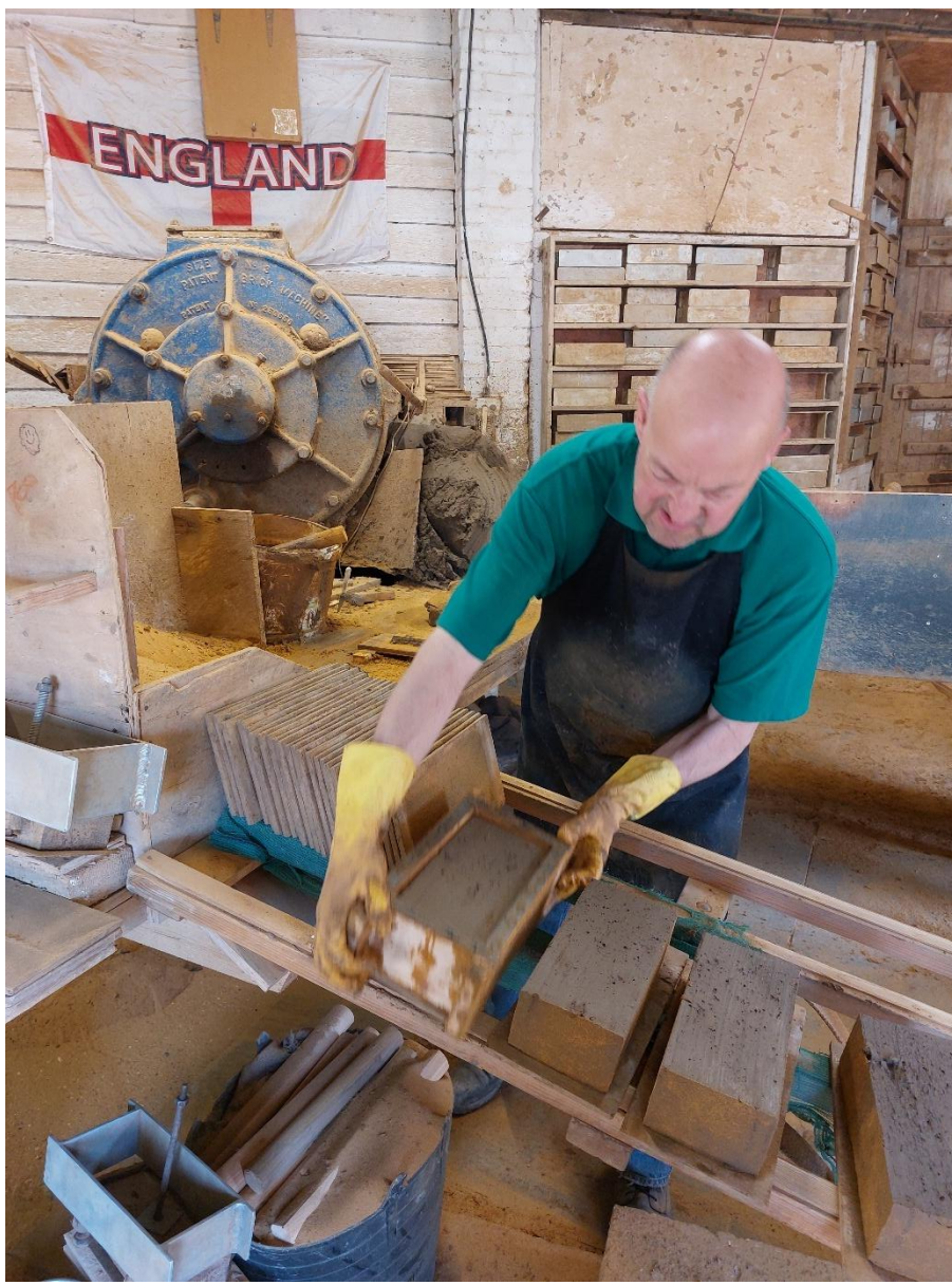
Making the bricks by hand (Photo. Louise Harrison)
